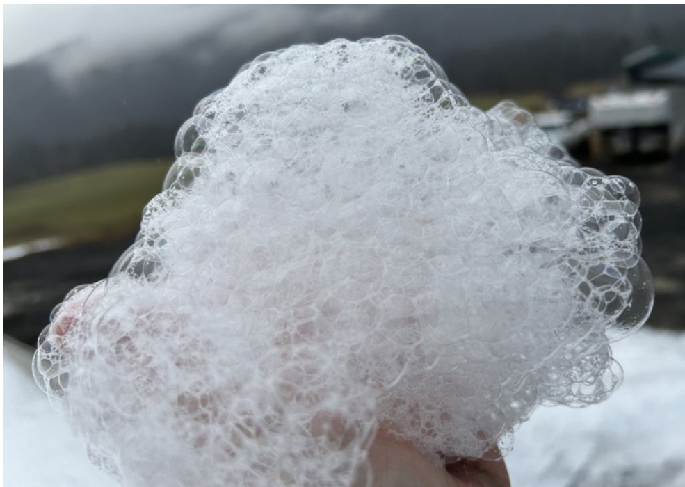
High-expansion nitrogen foam uses large, dry bubbles to create an oxygen-free environment.
